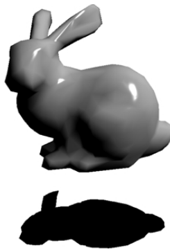
FIGURE 55. The Stanford bunny model with a planar shadow created by linear transformations
