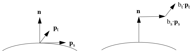
FIGURE 119. Bump mapping. The normal vector is modified by components in u and v direction
