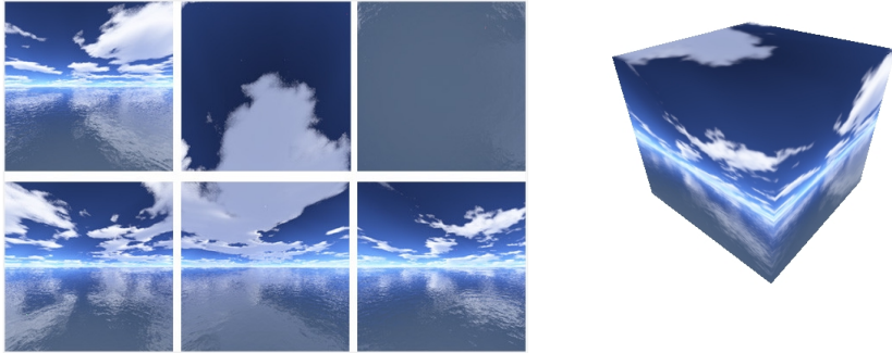
FIGURE 113. A nice skybox texture, shown as six separate textures and mapped onto a cube.
