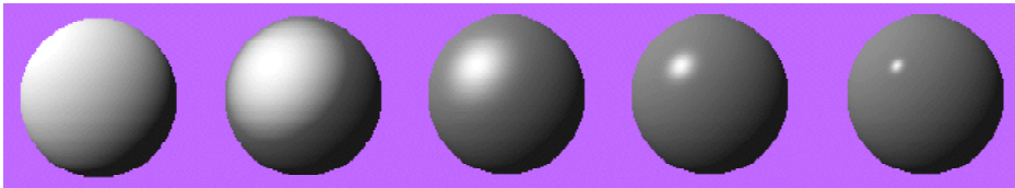
FIGURE 42. Shading of a sphere with diffuse reflection (far left) and specular reflection with shininess \alpha = 1, 5, 25 and 125 (remaining four).
