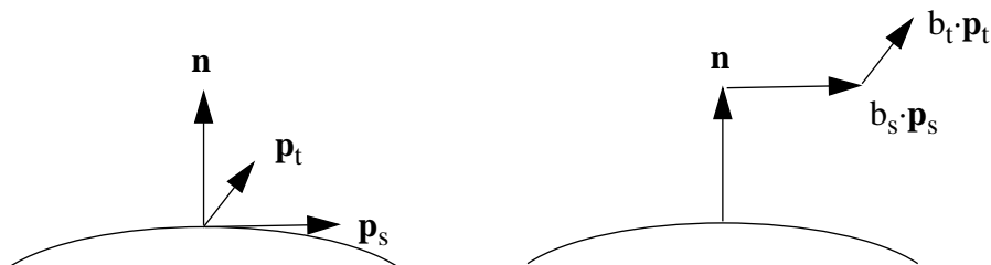
FIGURE 121. Bump mapping. The normal vector is modified by components in u and v direction
