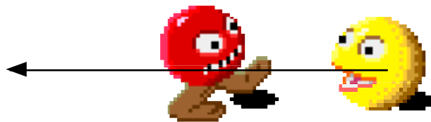
FIGURE 173. If the movement per cycle is too big, objects run a risk of passing through each other
