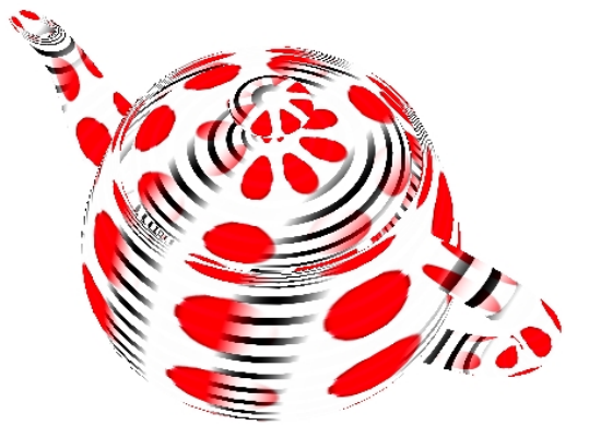
FIGURE 112. Multitextured Utah teapot, mixing two textures in the fragment shader
