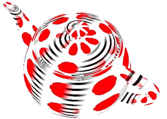
FIGURE 108. Multitextured Utah teapot, mixing two textures in the fragment shader
