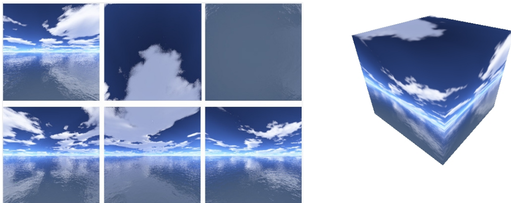
FIGURE 111. A nice skybox texture, shown as six separate textures and mapped onto a cube.
