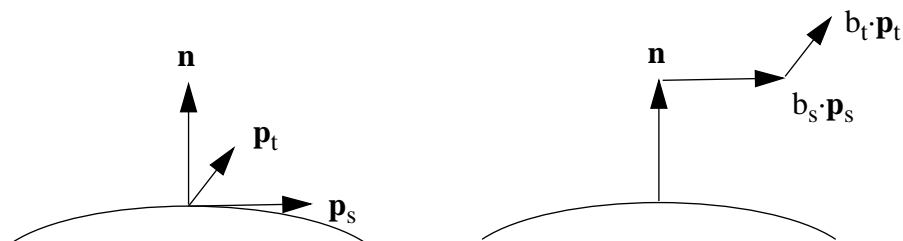
FIGURE 117. Bump mapping. The normal vector is modified by components in u and v direction
