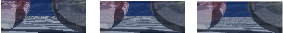
FIGURE 215. Ray-traced image, detail. Left: no anti-aliasing. Middle: 2x2 super-sampling. Right: 2x2 distributed ray-tracing, 4 random rays
