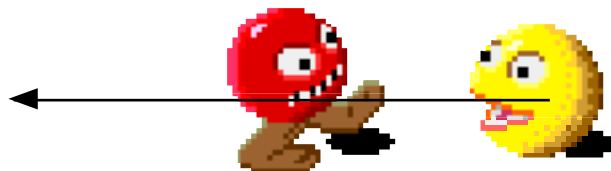
FIGURE 169. If the movement per cycle is too big, objects run a risk of passing through each other
