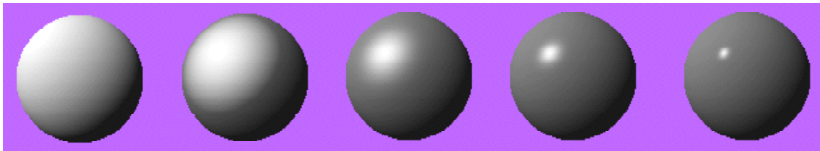
FIGURE 45. Shading of a sphere with diffuse reflection (far left) and specular reflection with shininess n = 1, 5, 25 and 125 (remaining four).
