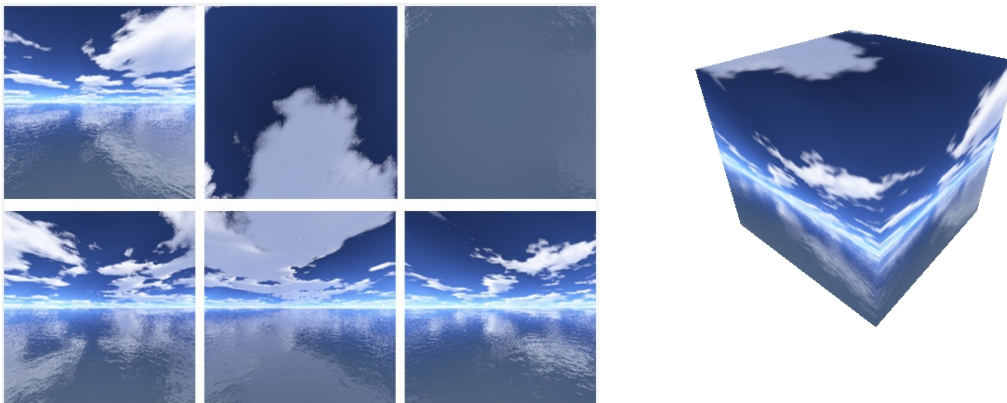
FIGURE 105. A nice skybox texture, shown as six separate textures and mapped onto a cube.
