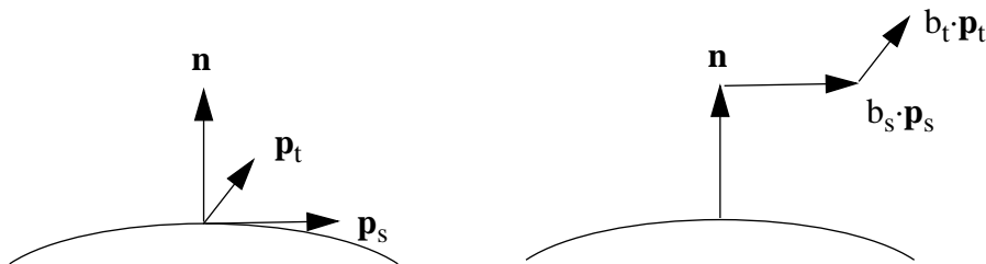
FIGURE 111. Bump mapping. The normal vector is modified by components in u and v direction
