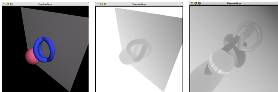
FIGURE 24. Rendering from the light source, image and Z buffer, and the Z buffer projected over the scene
