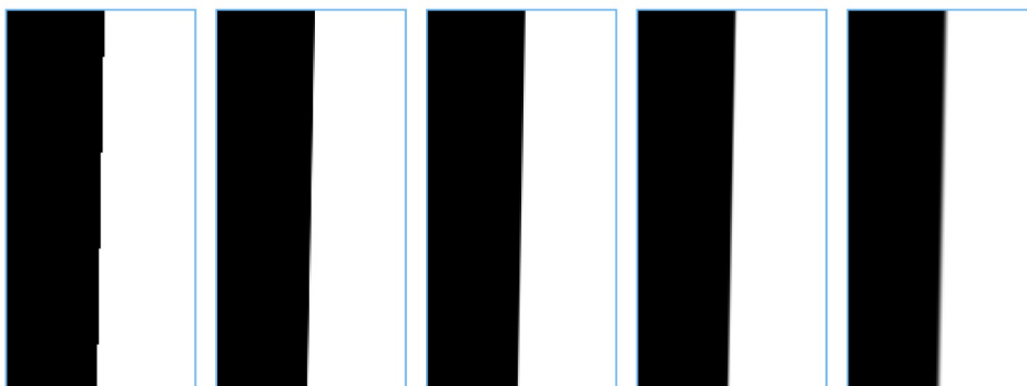
Edges using smoothstep with different step widths in proportion to \|\nabla F\| . From left to right: 0.0, 1.0, 1.5, 2.0, 4.0.
