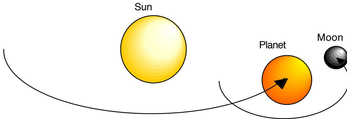
The sun is drawn at  $x_s, y_s, z_s$ , the planet rotates around the sun at radius  $r_p$ , with the angle  $a$ , and also rotates around its own Y axis by the angle  $b$ . Similarly, the moon rotates around the planet at radius  $r_m$ , angle  $c$ , and rotates around its Y axis by angle  $d$ .
