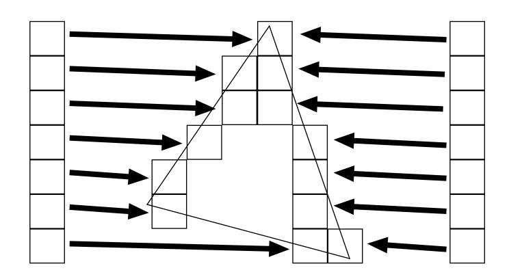
Write edges to span-buffer, then fill each interval
