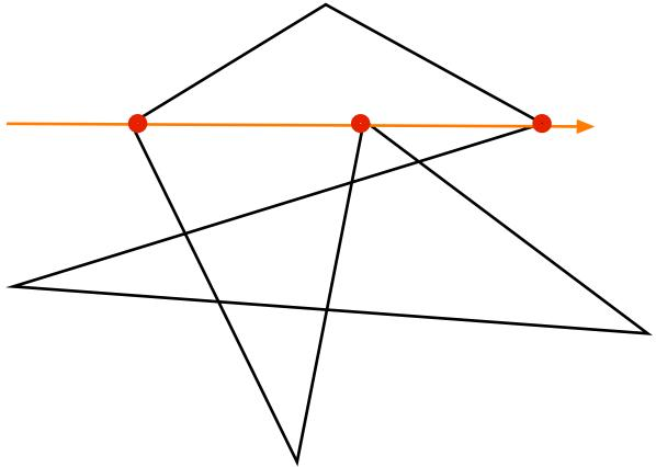
We get a count of two at each, which causes incorrrect filling!
