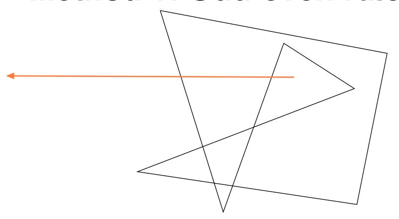
To learn if a pixel is inside the polygon, you can apply the same kind of test!
