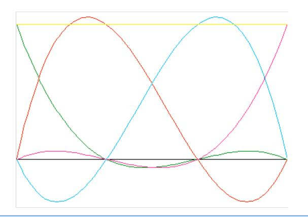
Actual blending functions for interpolated spline of 4 control points (similar to Bézier)
