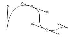
Originally a drafting tool to create a smooth curve
