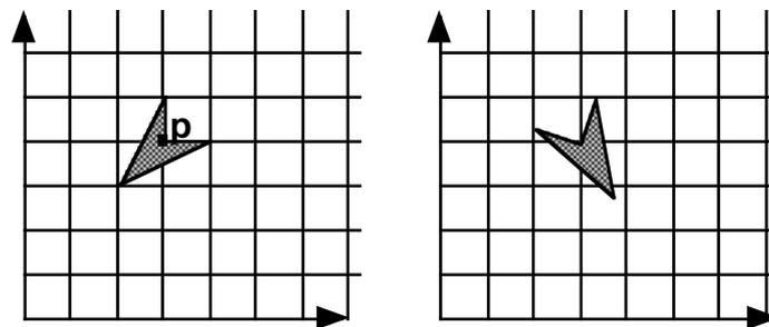
Original shape and position, and the point  $\mathbf{p}$  that the shape is rotated around
